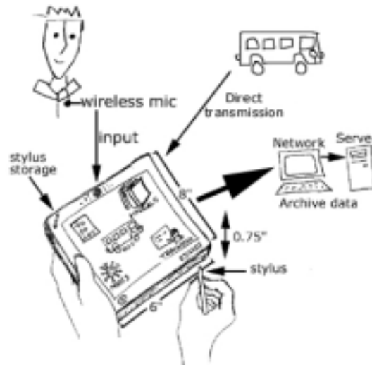
Figure 1. An example of a handheld wireless EPSS with a GUI design, wireless microphone, and stylus.
